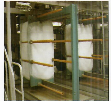
Fig. 5 Due to flexible design, no damage will occur when freezing.
